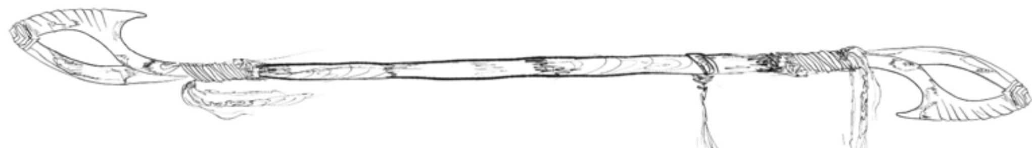
A device to avoid getting lost in snow storms or heavy blizzards – one person walks in front, grabbing the front handle while another walks in the back. The handles are not located on the same side in order to not block the view.
